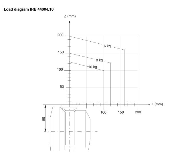
1.5.2 Maximum load and moment of inertia for full and limited axis 5 movement
